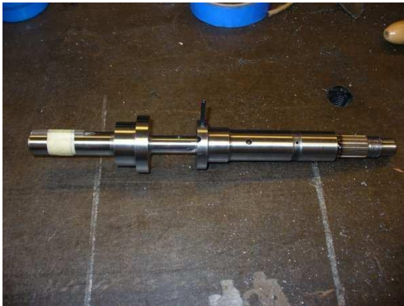
Figure 13: Completed Machined Crankshaft
